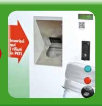
The automatic identification optional module allows the bar-code reading of the waste introduced inside the machine.
